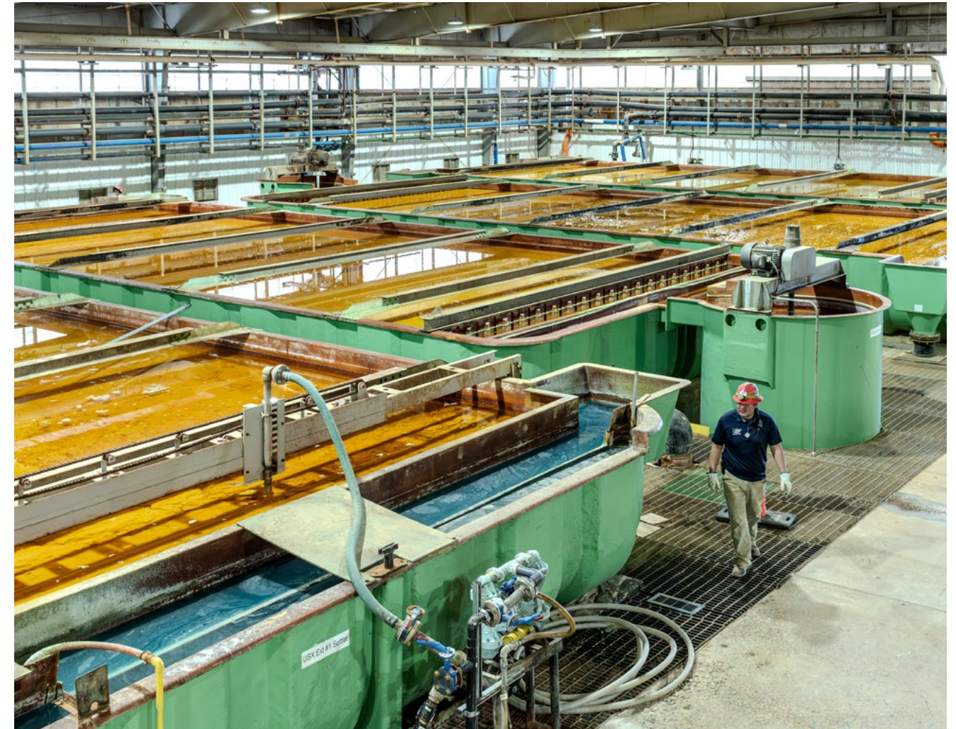
Processing infrastructure at the White Mesa Mill enables Energy Fuels to recover uranium, vanadium, and rare earth elements as part of its “targeted recycling” approach to critical mineral production.
