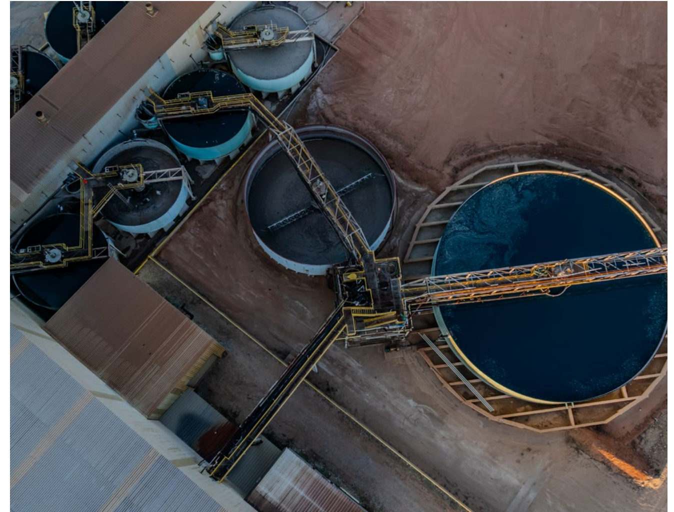
Aerial view of processing tanks and thickeners at White Mesa Mill, part of Energy Fuels' operations recovering uranium, rare earth elements, and other critical materials.
