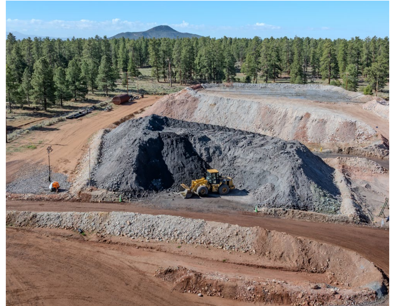
Uranium ore stockpile at the Pinyon Plain Mine, processed into uranium oxide (U 3 O 8 ) for powering carbon-free nuclear energy.
