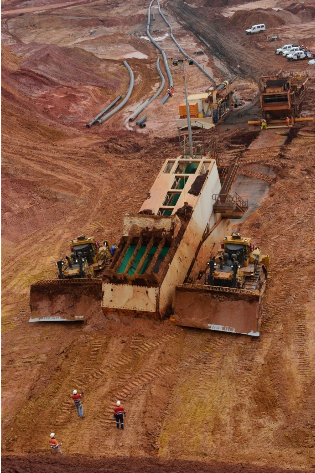
Figure 16-4: Dry mining unit relocation
