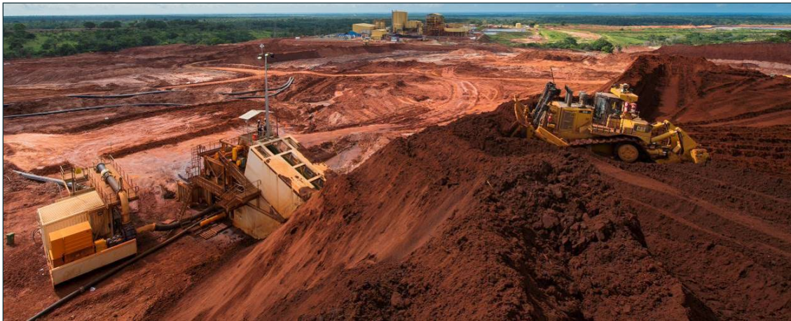
Figure 15-4: Dry mining dozer push
