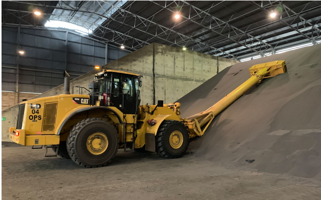
Figure 18-10: Typical FEL stacking with pusher blade
