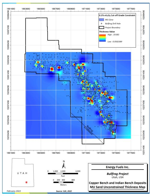
Figure 14-6: Copper Bench and Indian Bench Deposits MU Sand Unconstrained Thickness Map
