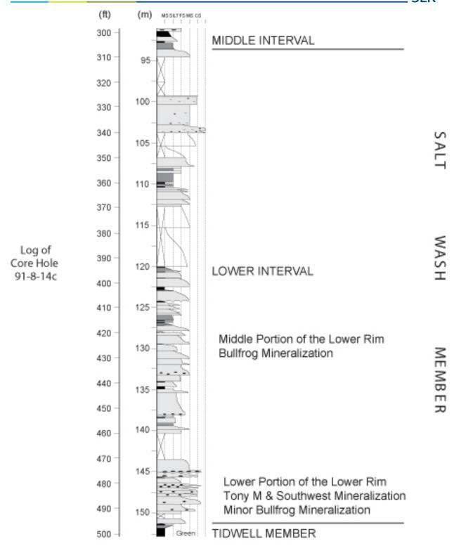
Figure 7-3: Detail of the Lower Portion of the Lower Rim of the Saltwash Member
