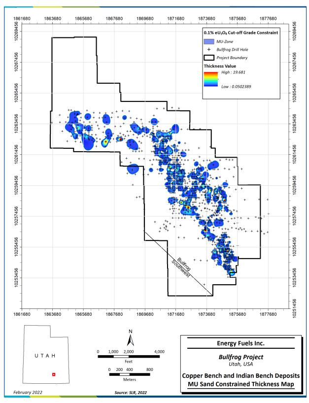
Figure 14-9: Copper Bench and Indian Bench Deposits MU Sand Constrained Thickness Map
