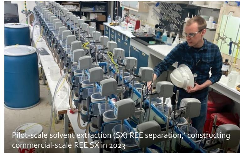
Pilot-scale solvent extraction (SX) REE separation, constructing commercial-scale REE SX in 2023
