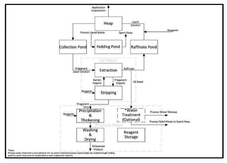
Figure 17-2. Heap Leach Process Block Flow Diagram
