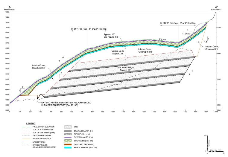
Figure 17-6. Heap Leach Reclamation Cover Cross-Section (A-A')
