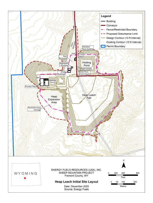
Figure 17-3. Heap Leach Initial Site Layout
