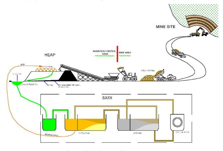
Figure 17-1. Typical Heap Leach Schematic
